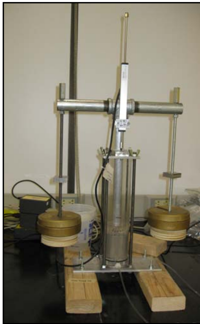
Figure 4: Resedimentation set up at unload.
