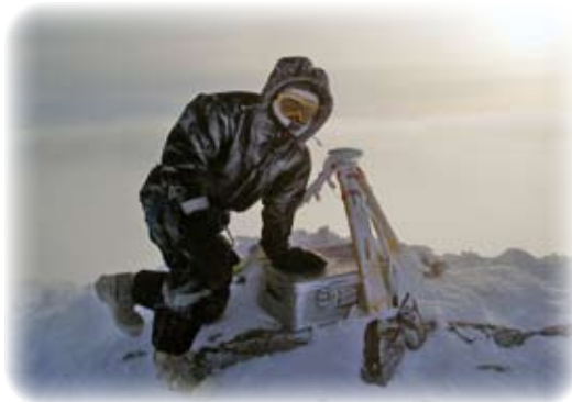
Peter Kuipers Munneke weathers a blizzard on Norway's Nordenskiöldbreen Glacier to install a GPS base antenna. Photo: Veijo Pohjola
