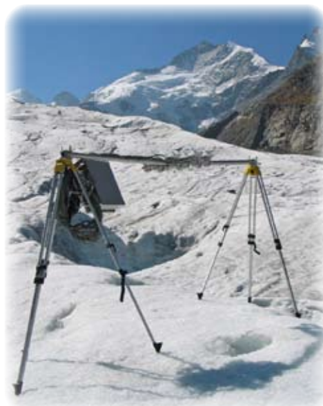
Peter uses a weather station like this to measure thermal and solar radiation, temperature, humidity, wind speed and direction, pressure and snow temperature. This unit is on the Greenland ice sheet, about 100 kilometers inland from Kangerlussuaq. Photo: Wim Boot
