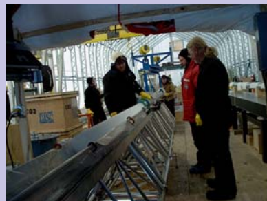
The team pushes the core out of the barrel. Photo: Kim Wolfe
